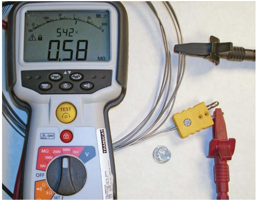
**Fig. 4. Room-temperature insulation resistance being tested using a “megger.” Note that this TC reads 999.42 megaohms LESS than the ASTM E608 minimum.**
