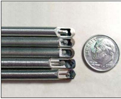
**Fig. 1. Only the top two TCs meet the ASTM E608 specification for “measuring junction configuration.”**
